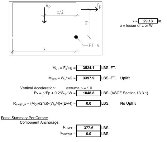
Anchors Embedded in Concrete or CMU:
